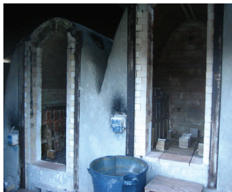
Susan's two chamber Anagama kiln
